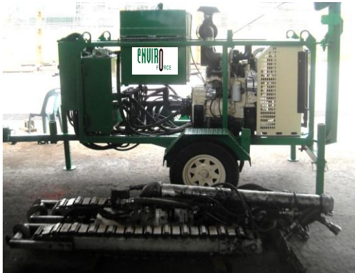
Remote Controlled Tank Cleaning Tractor c/w onboard pump www.enviroforce.com
